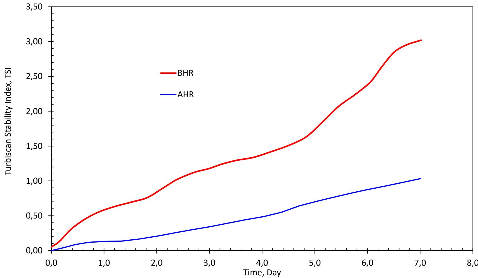
The higher the TSI, the faster particles settle in the sample fluid.
